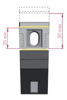
Shelf is clamped between a layer of ridged plastic on the lower side and soft rubber on the upper side (coloured parts).
